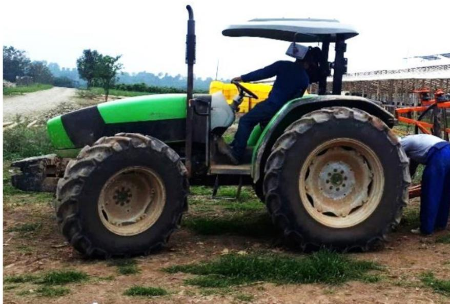
Fig. 2. Tractor Deutz-Fahr Agrofarm 420-T Ecoline.
