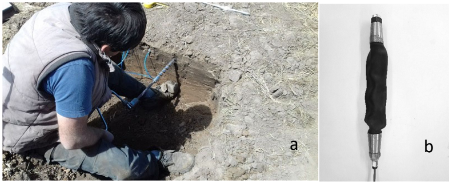
Fig. 1. Installation of pressure probes in the soil profile through a test pit (a), and detailed view of the pressure probe acting as an interface between the soil and the electronic pressure transducer (b).
